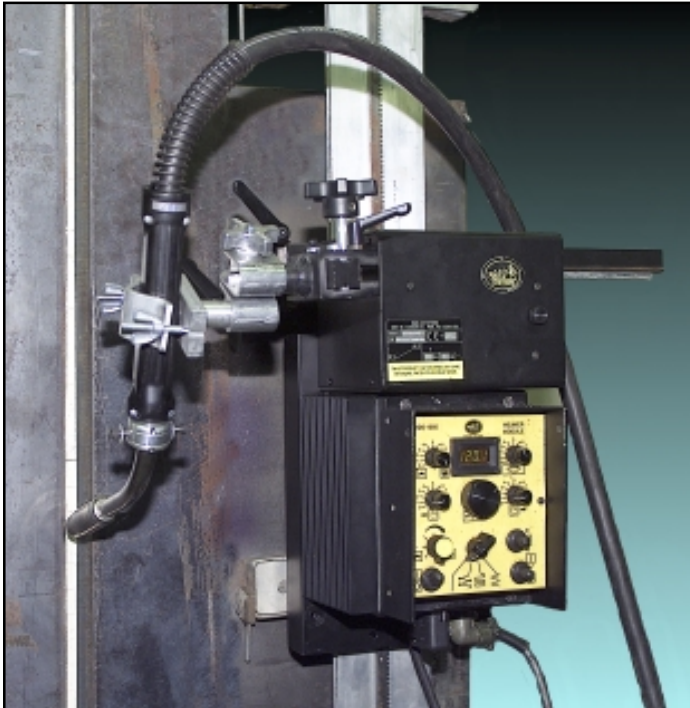
One-sided welding with Bug-O Systems MDS Travel Carriage.
